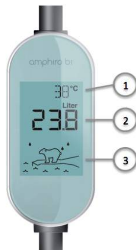
Figure 2: Schematic representation of the feedback device amphiro b1
