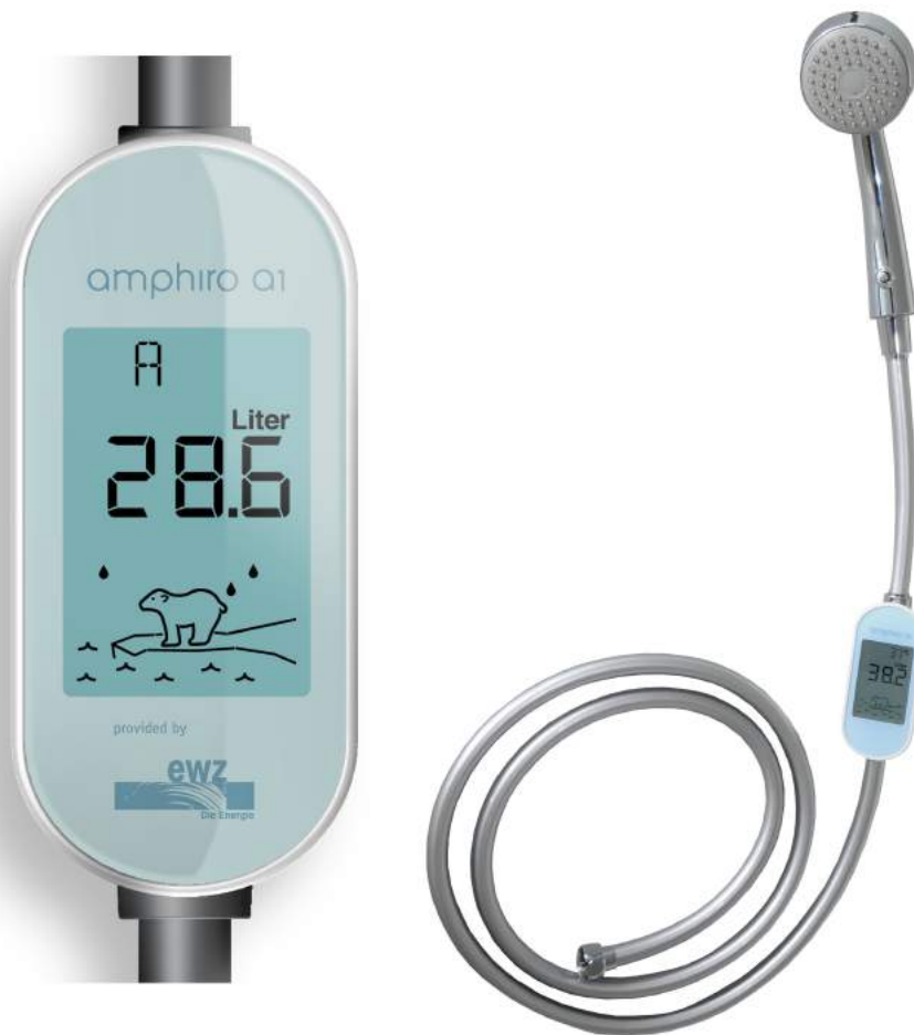
Figure 3.1: On the left: amphiro a1 display and body; on the right: the device installed between showerhead and showerhose
